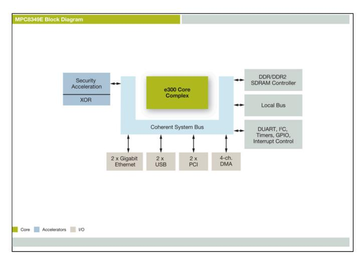
View additional information for PowerQUICC® II Pro Processor with DDR2, Dual PCI, 1 GB Ethernet, Dual USB, Security.
