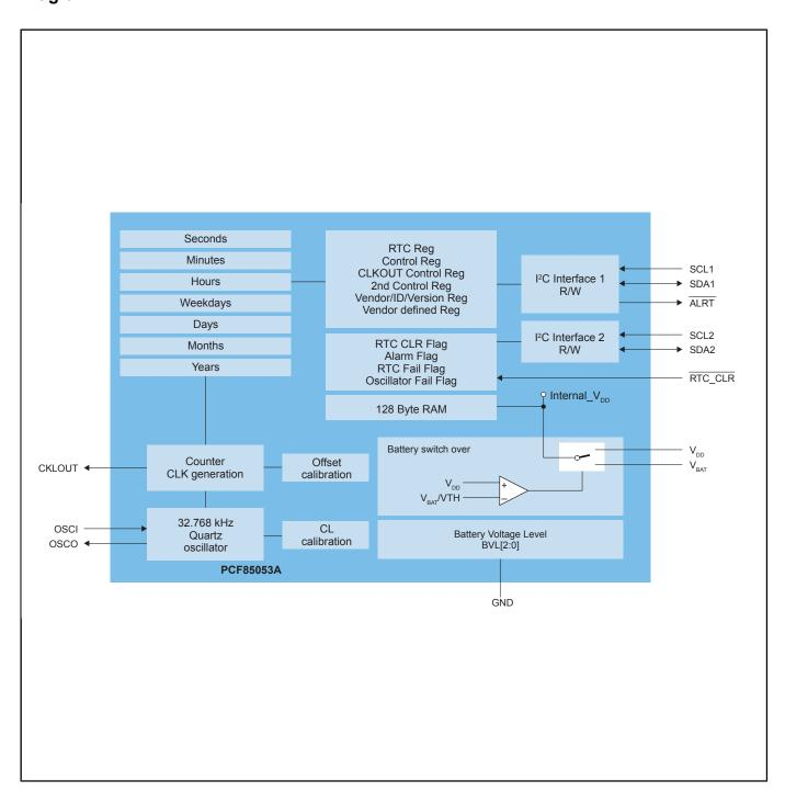
View additional information for Bootable CPU RTC with Two I<sup>2</sup>C Buses, 128 Byte SRAM and Alarm Function.
