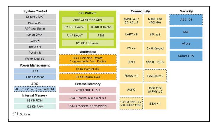
View additional information for i.MX 6ULL Single-Core Processor with Arm® Cortex®-A7 Core.
