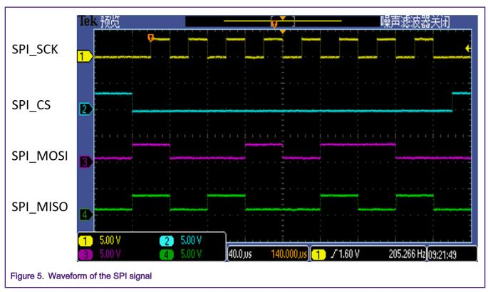
The SPI master board sends 0x96 to the SPI slave board and receives 0xa5 at the same time. Figure 6shows the communication data between SPI master and slave.
