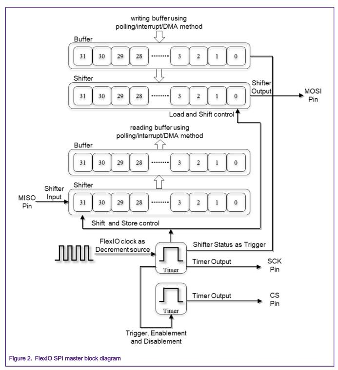
In this application note, Timer 0 generates SPI\_SCK signal and outputs to FlexIO\_D26, Timer 1 generates SPI\_CS signal and outputs to FlexIO\_D0, Shifter 0 connects to FlexIO\_D21 to transmit the data on each rising edge of SPI\_SCK, Shifter 1 connects to FlexIO\_D22 to receive the data on each falling edge of SPI\_SCK. Table 1 shows the configuration for Timer 0.
