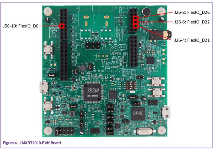
In this application, FlexIO\_D21 pin as data output pin, FlexIO\_D22 pin as the data input pin, FlexIO\_D26 pin as the SPI\_SCK, and FlexIO\_D0 pin as SPI\_CS.
