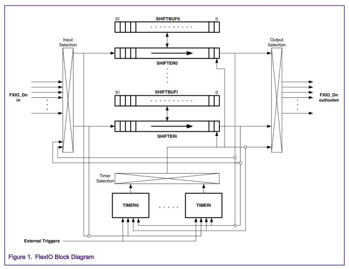
From the FLEXIO\_PARAM register, users can read the amount of these resources like shifter, timer, pin, and trigger. For instance, there are eight shifters, eight timers, 32 pins, and two external triggers in I.MXRT1010 (In this device, limited by the number of pins, FlexIO only has 27 pins).
