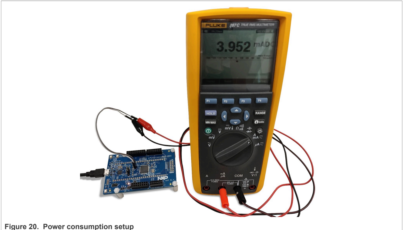
Figure 20. Power consumption setup
