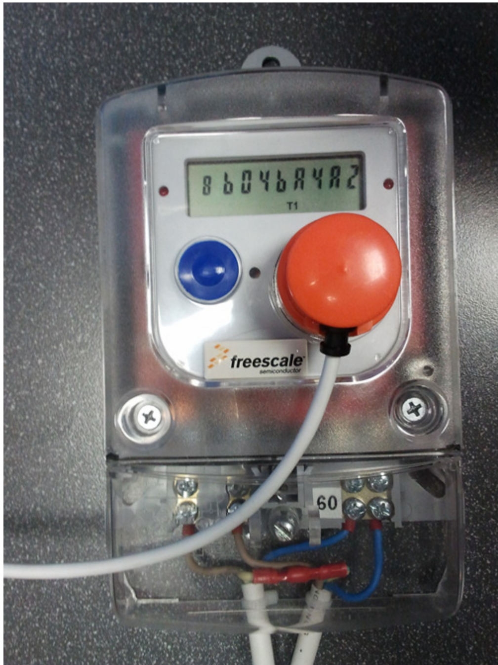
Figure 8. Single-phase power meter with ripple control receiver functionality displays a received ripple control message on September 24th, 2015, at 3:51 p.m. in Roznov pod Radhostem in hexadecimal format.
