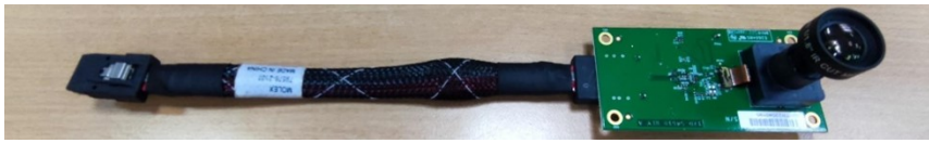
Figure 21. OS08A20 CSI MIPI camera
