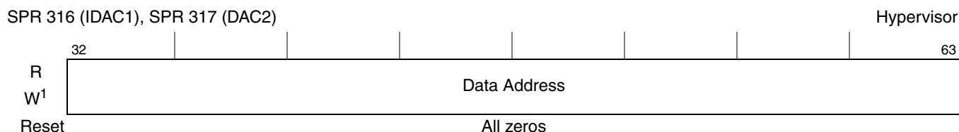
Figure 2-46. Data Address Compare Registers (DAC1–DAC2)
