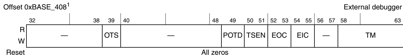
Figure 9-7. Nexus Development Control Register 1 (DC1)
