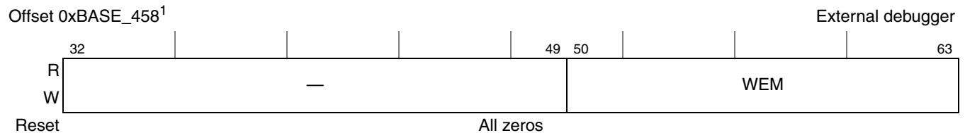
Figure 9-11. Nexus Watchpoint Mask Register
