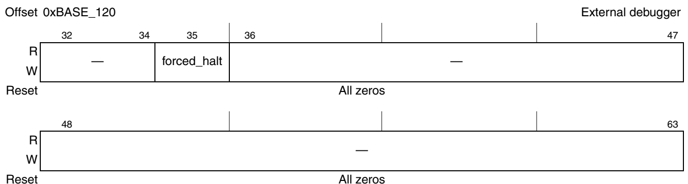
Figure 9-6. Extended External Debug Control Register 0 (EEDCR0)
