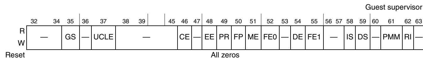
Figure 2-1. Machine State Register (MSR)
