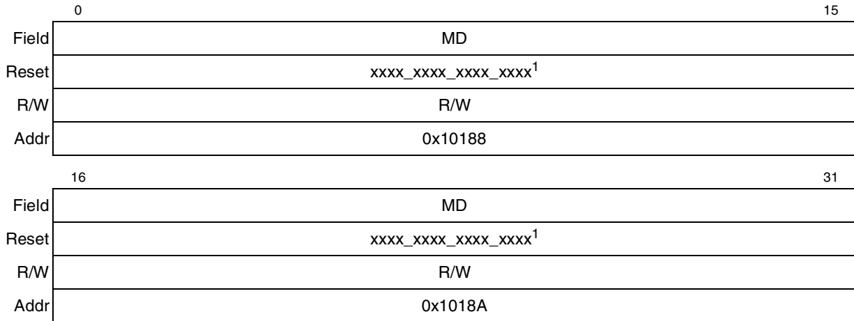
Figure 11-12. Memory Data Register (MDR)
