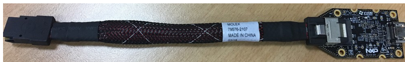
Figure 9. i.MX mini SAS cable with DSI-to-HDMI adapter
