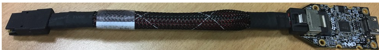
Figure 14. i.MX mini SAS cable with LVDS-to-HDMI adapter
