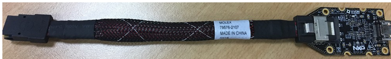
Figure 18. i.MX mini SAS cable with DSI-to-HDMI adapter
