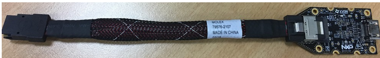
Figure 13. i.MX mini SAS cable with DSI-to-HDMI adapter
