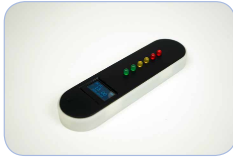
Figure 5. LPC8N04 MCU-based NFC Clock Demo Case
