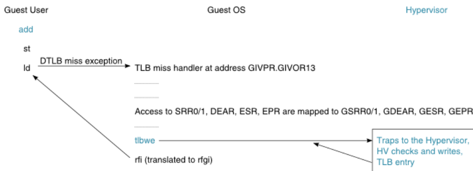
Figure 7. TLB exception handling by Guest-OS under Hypervisor control
